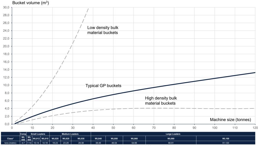
The machine size classes are based on the machine operating weight. Please consult the wheel loader producers for the latest information. Version 230413. © Copyright by SSAB 2000-2023.
