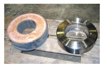
Crane steering wheels in a steel plate rolling mill. The wheels are normally changed every 3-5 years. Previously 35CrNiMo14 (similar to W.Nr.1.6582) machine steel was used. The wheels were induction-hardened to a depth of 10 mm. Now Toolox® 44 with no surface treatment is used. A major advantage in manufacturing is achieved since time is saved due to no need for heat treatment. Furthermore, cutting the rings from plate saved machining time and quaranteed a homogeneous small grain structure.
