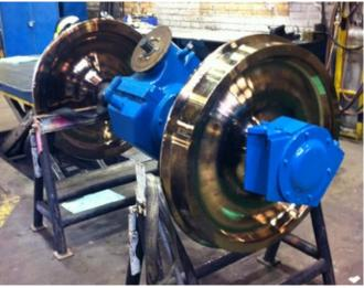
Wheels used in a steel coking plant locomotive. Previously the wheels were made from forged steel, which was a solution that worked well. The disadvantage was the long lead times once the wheels needed to be replaces. Making the wheels out of Toolox® 44 plates solved the problem.
