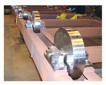
Toolox® maintains a high mechanical resistance up to 600°C. This is a benefit used in a wagon at an aluminium plant for charging aluminium coils into an annealing oven. The oven maintains a temperature at 560°C, which means that the wheels are repeatedly heated and cooled. Previous material for these wheels was stainless steel, now they have changed to Toolox® 44. Toolox® 44 retained it's mechanical properties longer when exposed to cyclic heating to 560°C.
