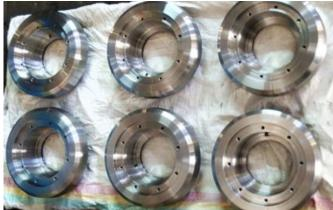
Guide rollers in cement mill stacker/reclaimer. In the previous solution, case-hardened 42CrMo4 was used. Changing to Toolox® 44 decreased the lead time with 10 days due to not needing to send the rollers for heat treatment. A much better surface finish with Toolox® gives better resistance to adhesive wear.
