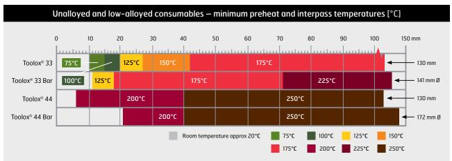
\*The tables are applicable to single plate thickness when welding with a heat input of 1,7 kJ/mm or more. For plate thicknesses not represented in the diagrams, contact SSAB for further information. If nothing else mentioned unalloyed and low-alloyed consumables apply.
