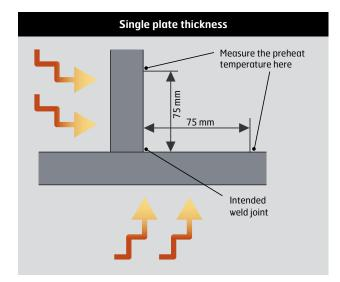
Measure the temperature of the thickest plate in the joint. A waiting time of minimum 2 min/25 mm thickness should be conducted before measuring the preheating temperature. The minimum preheating temperature should be obtained in an area of 75+75 mm around the intended weld joint.
