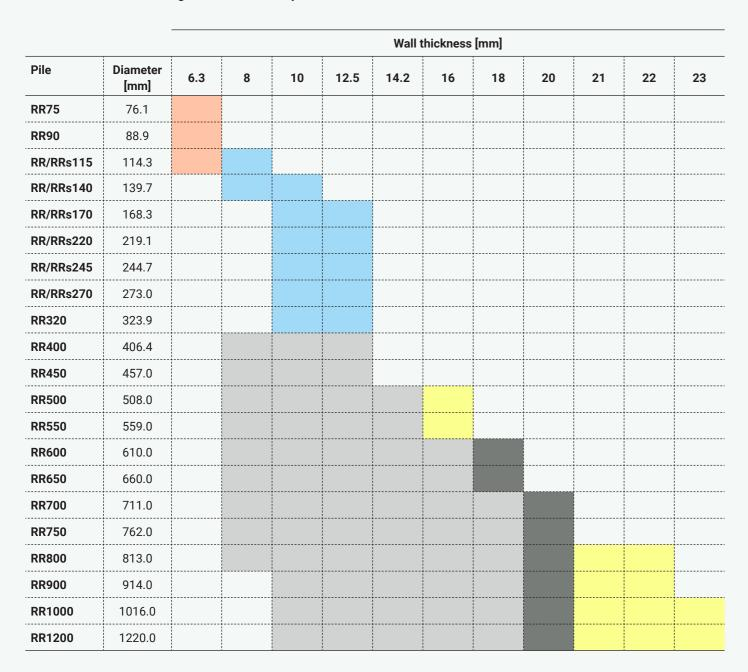
Table 3. Pile sizes and steel grades for drilled RD piles
