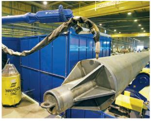
For instance, the manufacture of rock shoes for large diameter RR piles and their welding onto piles under workshop conditions using precise preheating of components and robotic welding equipment ensure the durability of weld seams and high and even quality of the end product.
