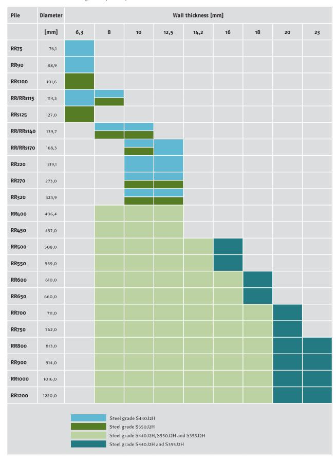
Table 3. Pile sizes and steel grades for RD piles.
