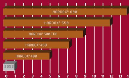
\*The calculations are based on sliding wear with steel scrap.
