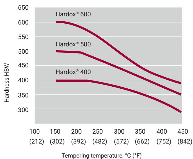
Figure 11: Surface hardness vs. tempering temperature.
