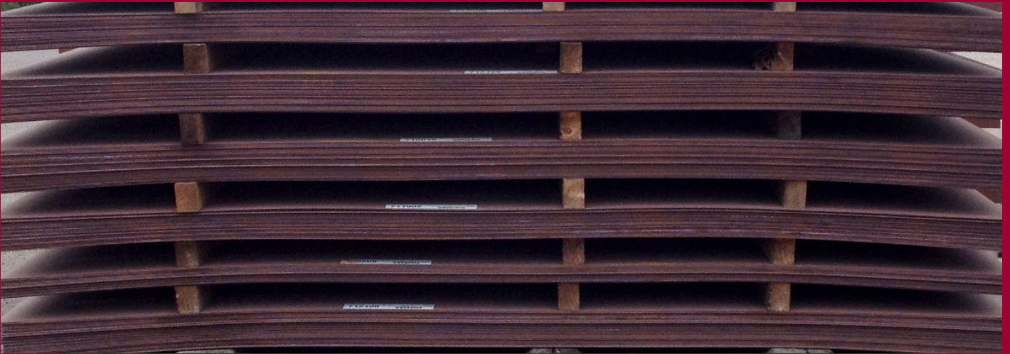
Figure 13a: Properly stacked plates.
