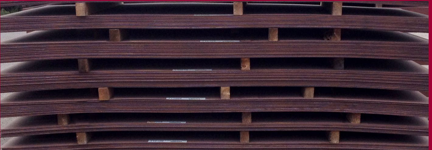
Figure 13b: Improperly stacked plates.
