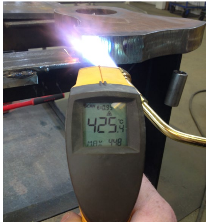
Figure 10: Temperature measurement during postheating.
