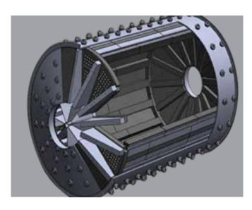
A rod mill is an application that requires significant wear resistance, as well as high crack resistance and toughness. In a rod mill bars are located inside a drum together with the mineral material, and the rotation crushes the minerals into smaller sizes.
