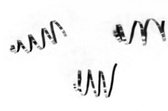
Slightly curled chips. Optimum feed
