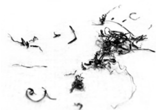
Thin or powdered chips. Increase feed
