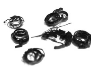
Thick, rough or burned chips. Reduce feed/ speed
