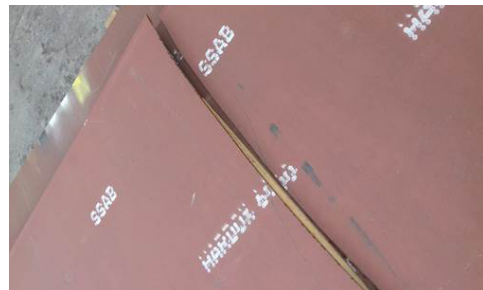
Example of a three-point force during storage.
