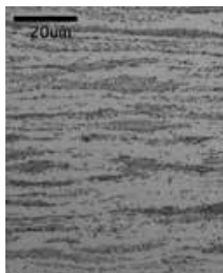
As-received cold rolled condition, ferrite and perlite.
