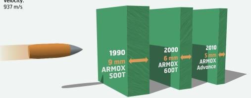
25 years of unparalleled product development, has made it possible to offer the market a protection plate that provides the same level of protection at half the plate thickness. This makes it possible to save 50 percent on weight, without compromising on safety. No one, can keep pace with our evolution.
