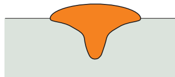
Fig. 12.6: The penetration profile promoted by a shielding gas with high argon content.
