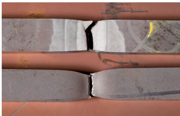
Fig. 7.2: The upper tensile test specimen includes a joint, while the lower specimen consists of unaffected parent metal.
