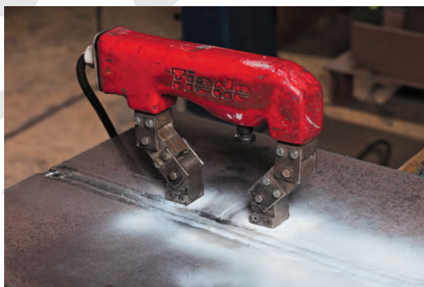
Fig. 18.3: Magnetization of a fillet joint with an electromagnet.
