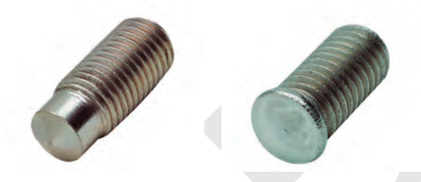
Fig. 19.3: The stud to the left is suitable for the drawn arc stud welding with ceramic ferrule or shielding gas. The stud to the right has a wide flange, which makes it appropriate to short cycle welding.
