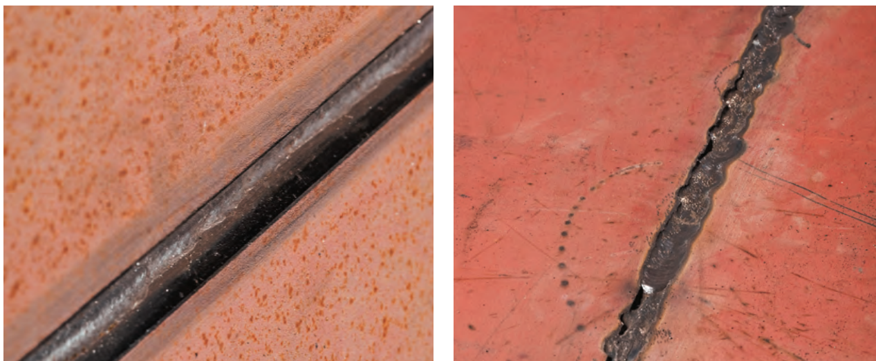
Fig. 14.13: A smooth weld geometry facilitates easier slag removal according to the picture on the left. An unsuitable performance from an unsteady welding performance is shown in the picture to the right.
