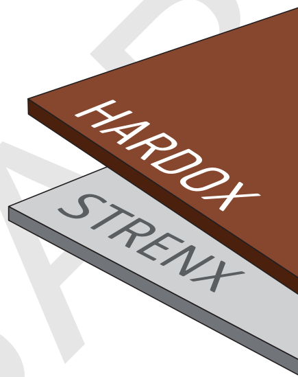
Fig. 9.1: The standard primer colors are red for Hardox and gray for Strenx.
