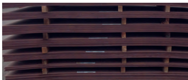
Fig. 11.13: Properly stapled plates.
