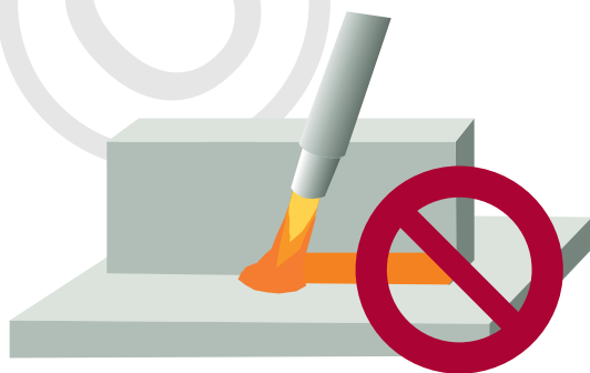
Fig. 4.11: Avoid start and stop sequences in corners when possible.
