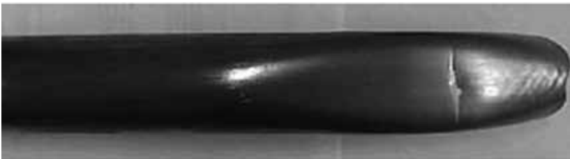
Figure 82. Tube bending defect: Mandrel seizing up with tube wall due to insufficient lubrication and wrong mandrel positioning and therefore breakage.
