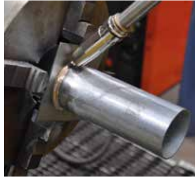
Figure 111. Arc brazing, flange joint.
