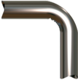
Figure 77. Excessive collapse with or without wrinkling throughout entire bend.
