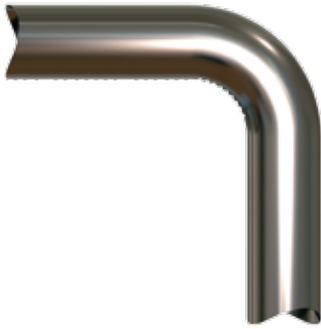
Figure 79. Wrinkles throughout bend area with wiper and mandrel in known position.
