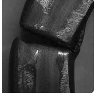
Figure 83. Tube bending defect: excessive tooling pressure and therefore scratching and breakage.
