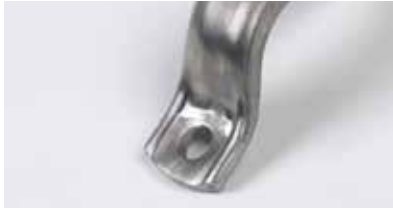
Figure 168. Flattened tube end. In connection with flattening, the end has been cut and/or punched.
