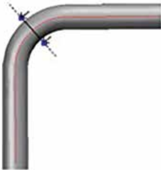
Figure 107a. Result of cross-section of stability indicating that the tube is still perfectly circular thanks to the mandrel used.
