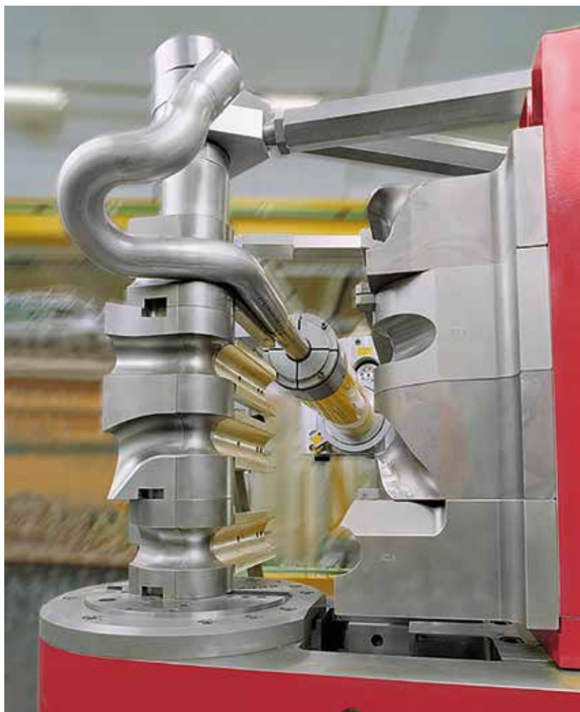
Figure 64. 3D bending with automated rotation. Courtesy of Herber Engineering AB.
