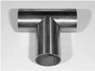
Figure 150. High precision tube joining “edge-to-edge” with curved surfaces.
