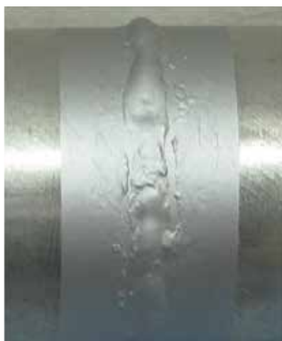
Figure 130. ARC-brazed joint of zinc-coated tube before (left) and after (right) salt spray test with zinc spray protection.
