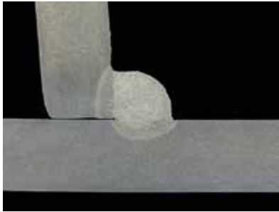
Figure 121. Excess weld metal.
