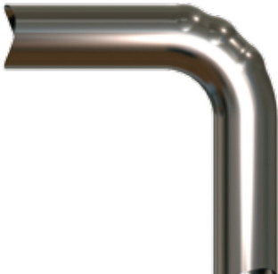
Figure 78. Mandrel ball humps.
