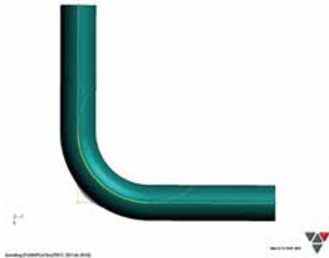
Figure 102. The tube of geometry, D=45\text{mm} , t=1.5\text{mm} and CLR=90\text{mm} , i.e. 2 \times D .
