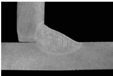
Figure 120. Excessive asymmetry of fillet weld
