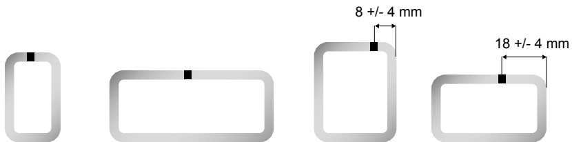
Figure 26. Possible weld seam positions and tolerances.
