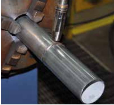
Figure 110. Arc brazing, butt joint.
