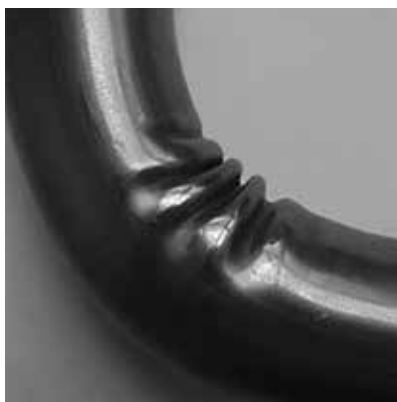
Figure 86. Tube bending defect: wrinkling due to extreme compression on inner radius.
