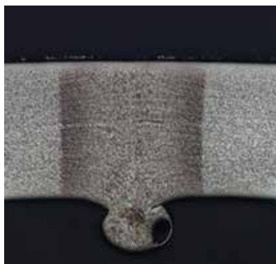
Figure 21. Example of a high-quality HF-weld: The edges are at the same level, and the inside burr shows there has been enough welding energy and squeeze pressure to create a quality weld.
