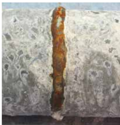
Figure 129. MAG-welded joint of zinc-coated tube after salt spray test without (left) and with zinc spray protection (right).
