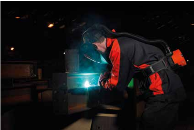
Figure 128. Fresh air helmet is use. Courtesy of Kemppi Oy.
