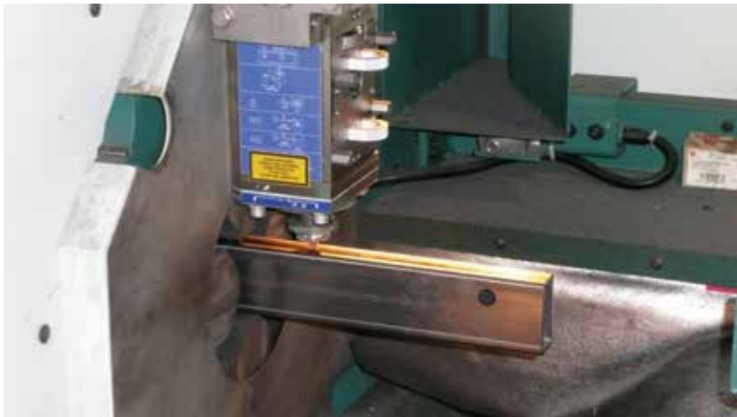
Figure 147. Centred tube by cutting head sensor. A separate measuring probe can also be used for centring.
