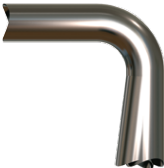
Figure 80. Bad mark at start of bend.
