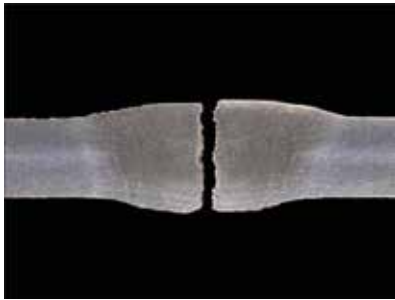
Figure 123. Cracks, e.g. hot crack.
