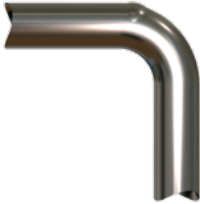
Figure 73. Hump at end of bend.
