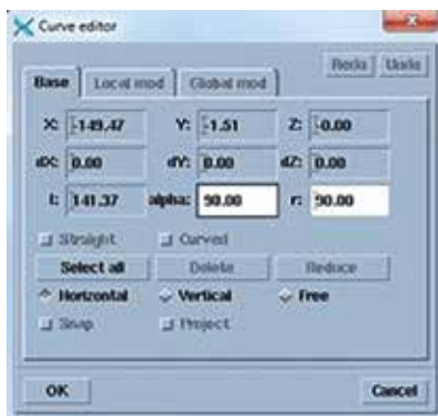
Figure 103. Parameter described in Figure above, additionally parameter l=141.37 mm, the length of the tube outside the bend.
