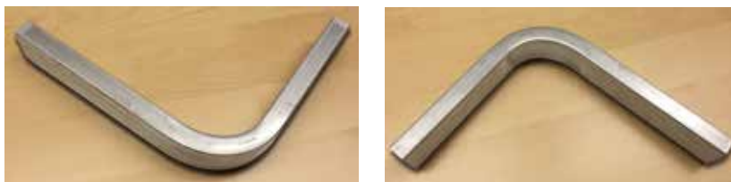
Figure 54. Bending square and rectangular sections.
