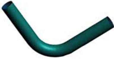
Figure 106a. The result obtained using a mandrel.
