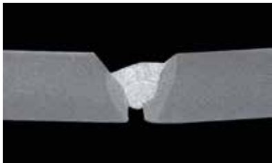
Figure 124. Lack of penetration.
