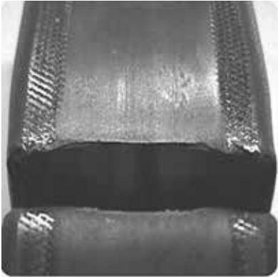
Figure 83. Tube bending defect: excessive tooling pressure and therefore scratching and breakage.
