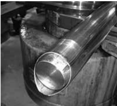
Figure 84. Tube bending defect: insufficient lubrication and therefore breakage.
