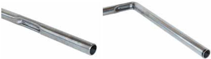
Figure 53. Decreasing bending radius by decreasing “D” of the tube.
