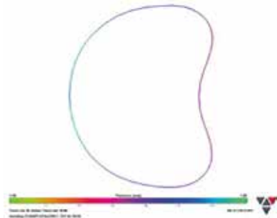
Figure 107b. The result of not using a mandrel, i.e. the cross-section has collapsed.
