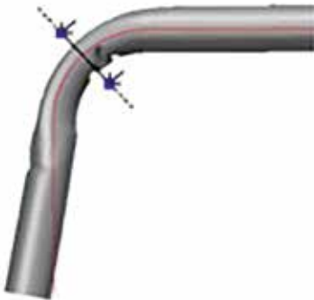
Figure 107b. The result of not using a mandrel, i.e. the cross-section has collapsed.
