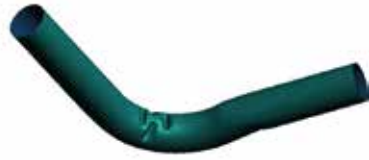
Figure 106b. The bend will collapse without mandrel.
