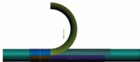
Figure 104. The die, wiper, pressure die and claws are shown.
