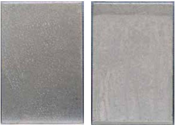
Figure 144. 24h in QCT 60°C. Left picture is Z600 and right one is hot dip galvanized.
