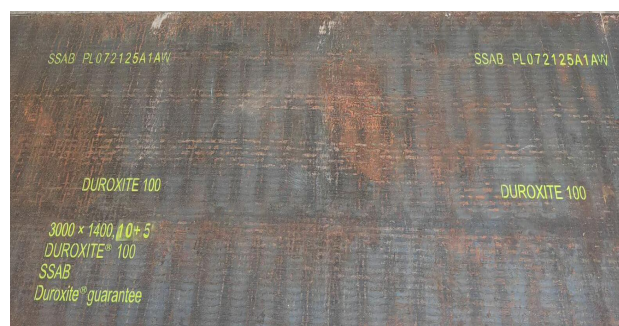
Example of marking on a Duroxite® overlay plate.
